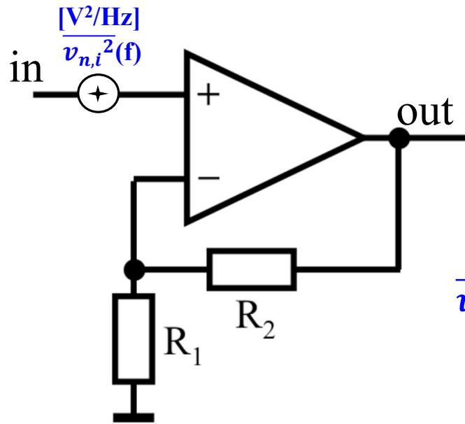
$$\overline{v_{n,i}^2}(R_1) = \left(4 \frac{nV}{\sqrt{\text{Hz}}}\right)^2$$
