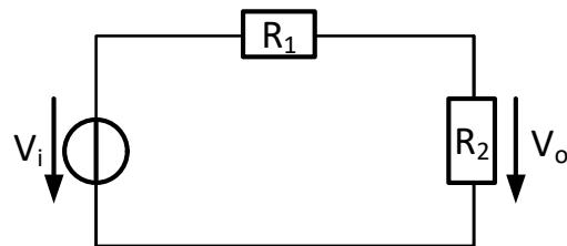
$$\overline{v_{n,o}^2}(f) = 4kT(R_1//R_2) = \frac{R_2 R_1}{R_2 + R_1} [V^2/Hz]$$
