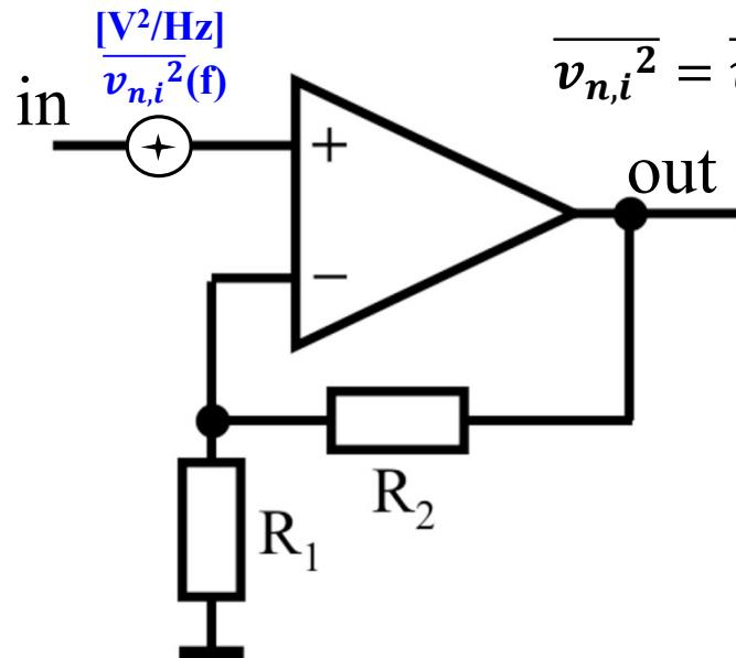
$$\overline{v_{n,i}^2} = \overline{v_{n,i}^2}(R_1) + \overline{v_{n,i}^2}(R_2) + \overline{v_{n,i}^2}(\text{Amp}) \approx \left(5 \frac{nV}{\sqrt{\text{Hz}}}\right)^2$$
